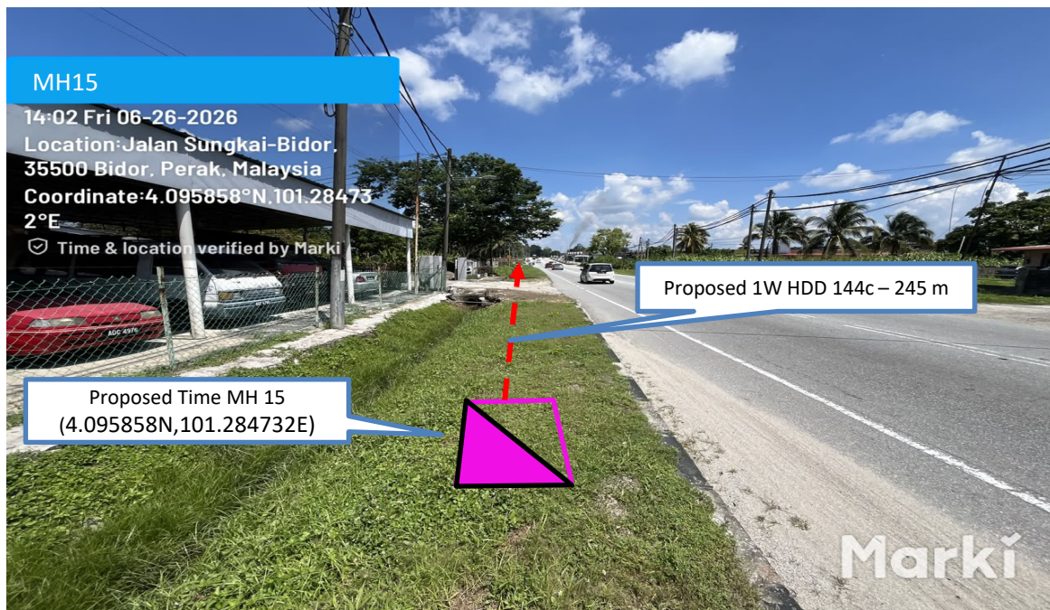
Prop 1W HDD 144C from Proposed Time MH15 n to Proposed Time MH16 – 245 m
