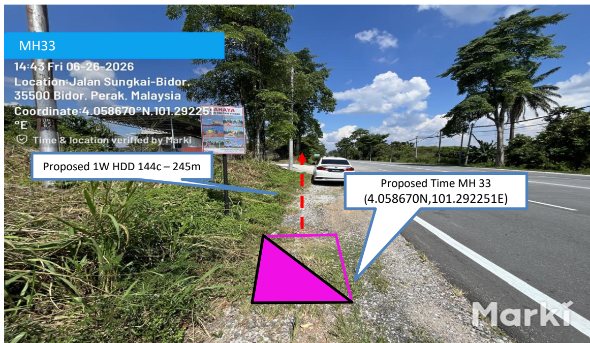
Prop 1W HDD 144C from Proposed Time MH33 to Proposed Time MH34– 245 m
