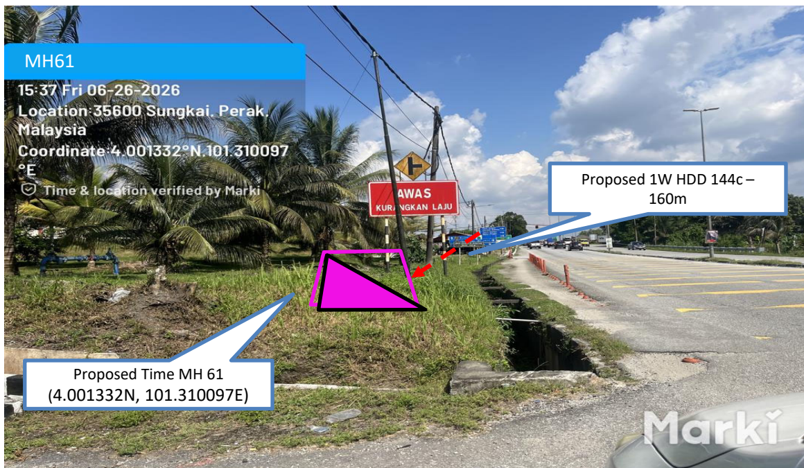
Prop 1W HDD 144C from Proposed Time MH61 to Proposed Time MH62– 160 m
