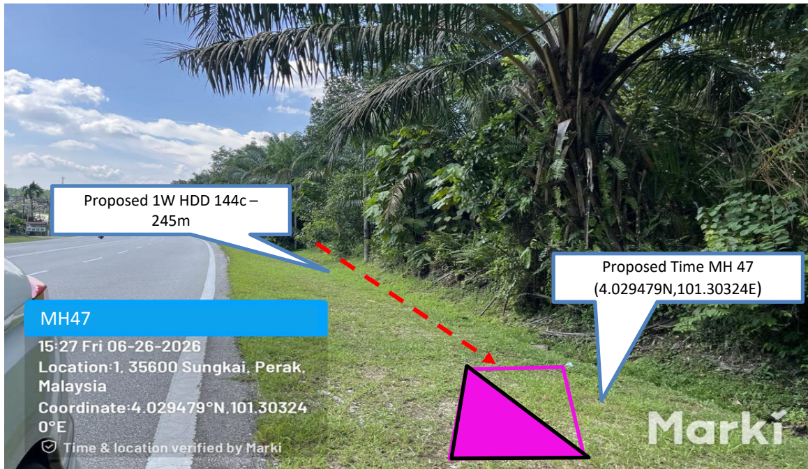
Prop 1W HDD 144C from Proposed Time MH46 to Proposed Time MH47–245 m
