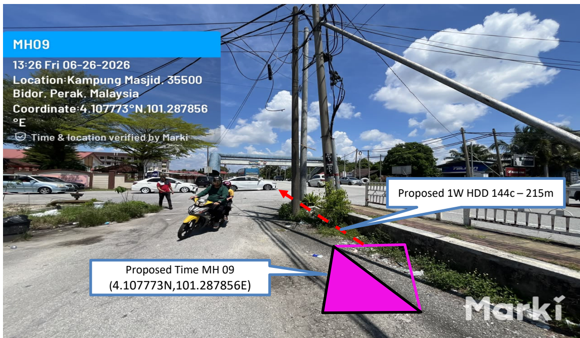
Prop 1W HDD 144C from Proposed Time MH09 n to Proposed Time MH10 – 215 m
