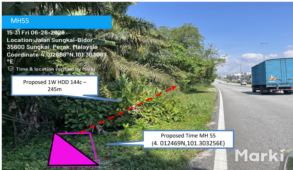
Prop 1W HDD 144C from Proposed Time MH55 to Proposed Time MH56– 245 m
