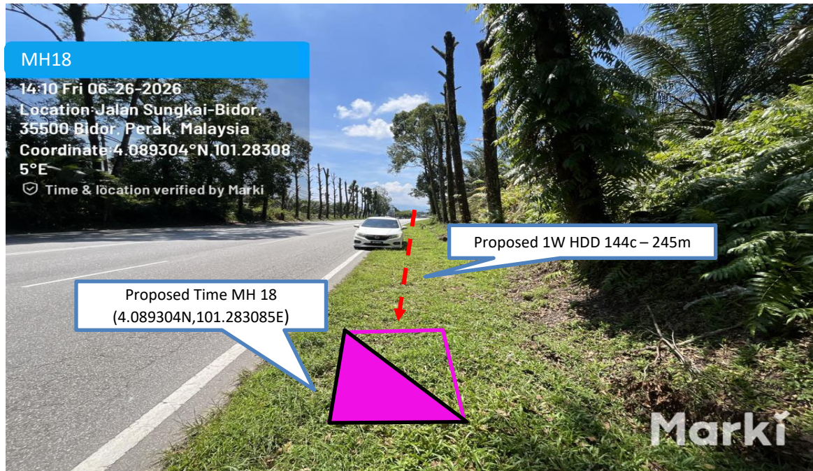
Prop 1W HDD 144C from Proposed Time MH17 to Proposed Time MH18 – 245 m
