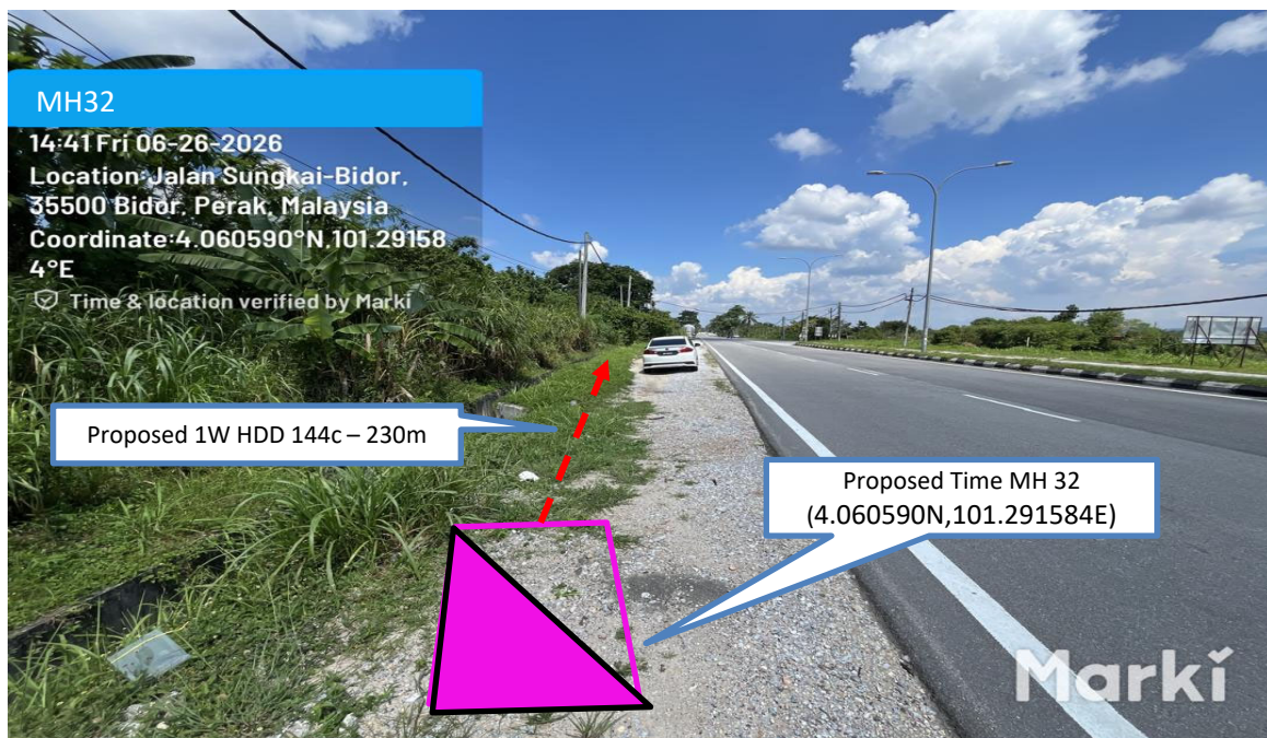
Prop 1W HDD 144C from Proposed Time MH32 to Proposed Time MH33– 230 m
