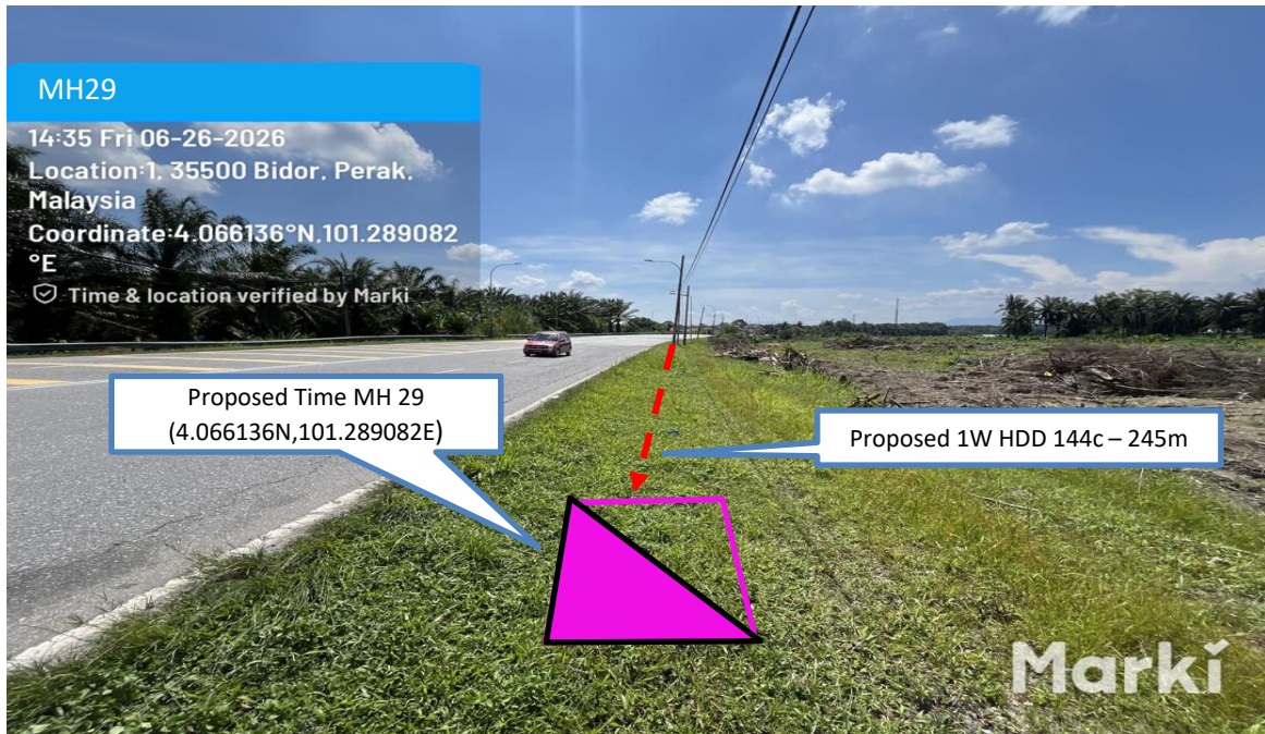
Prop 1W HDD 144C from Proposed Time MH28 to Proposed Time MH29 – 245 m
