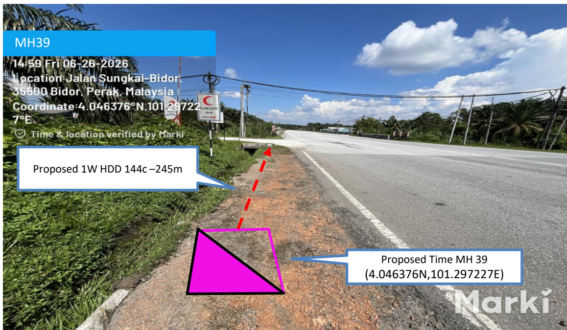
Prop 1W HDD 144C from Proposed Time MH39 to Proposed Time MH40– 245 m
