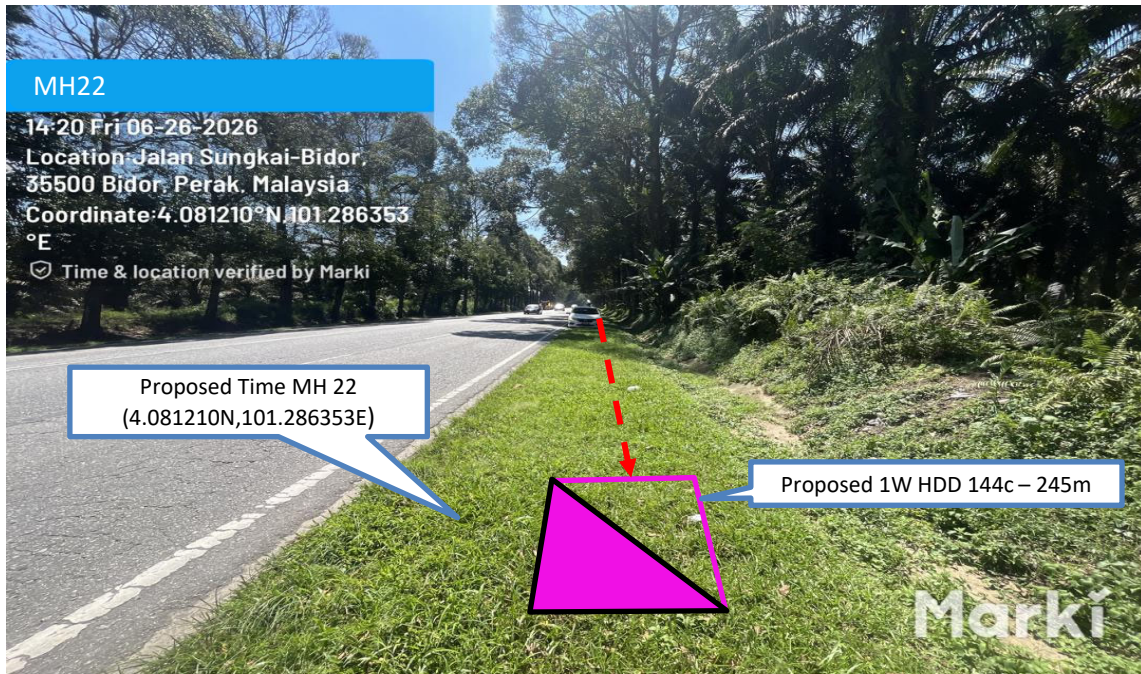
Prop 1W HDD 144C from Proposed Time MH21 to Proposed Time MH22 – 245 m
