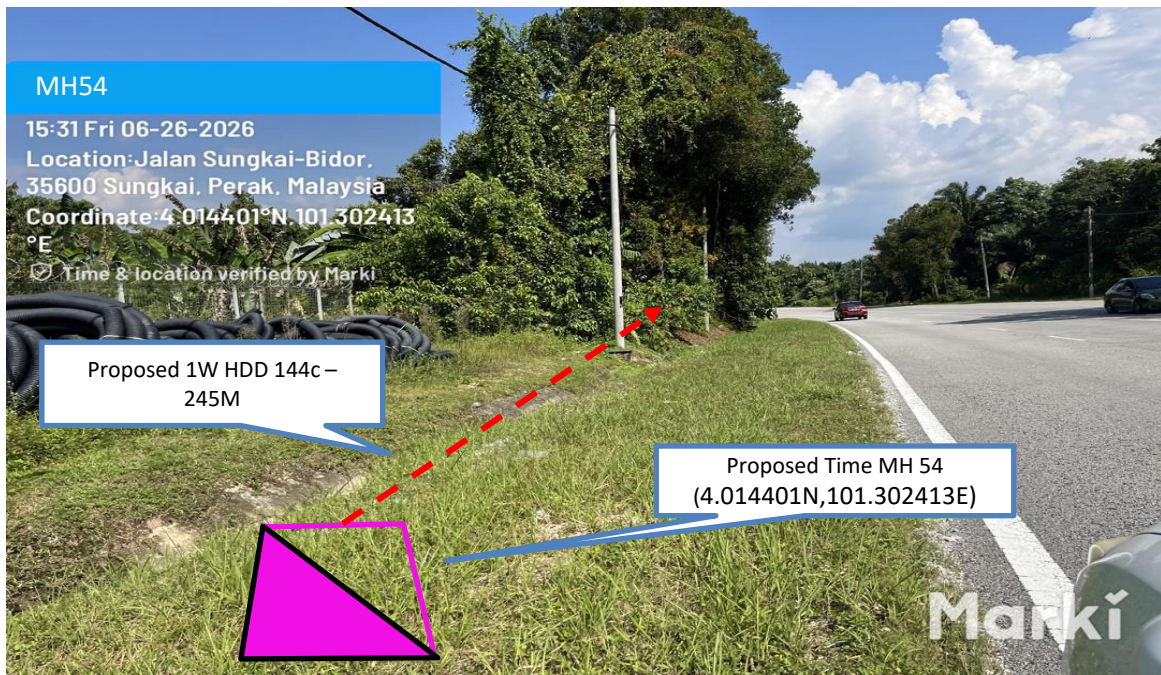
Prop 1W HDD 144C from Proposed Time MH54 to Proposed Time MH55– 245 m
