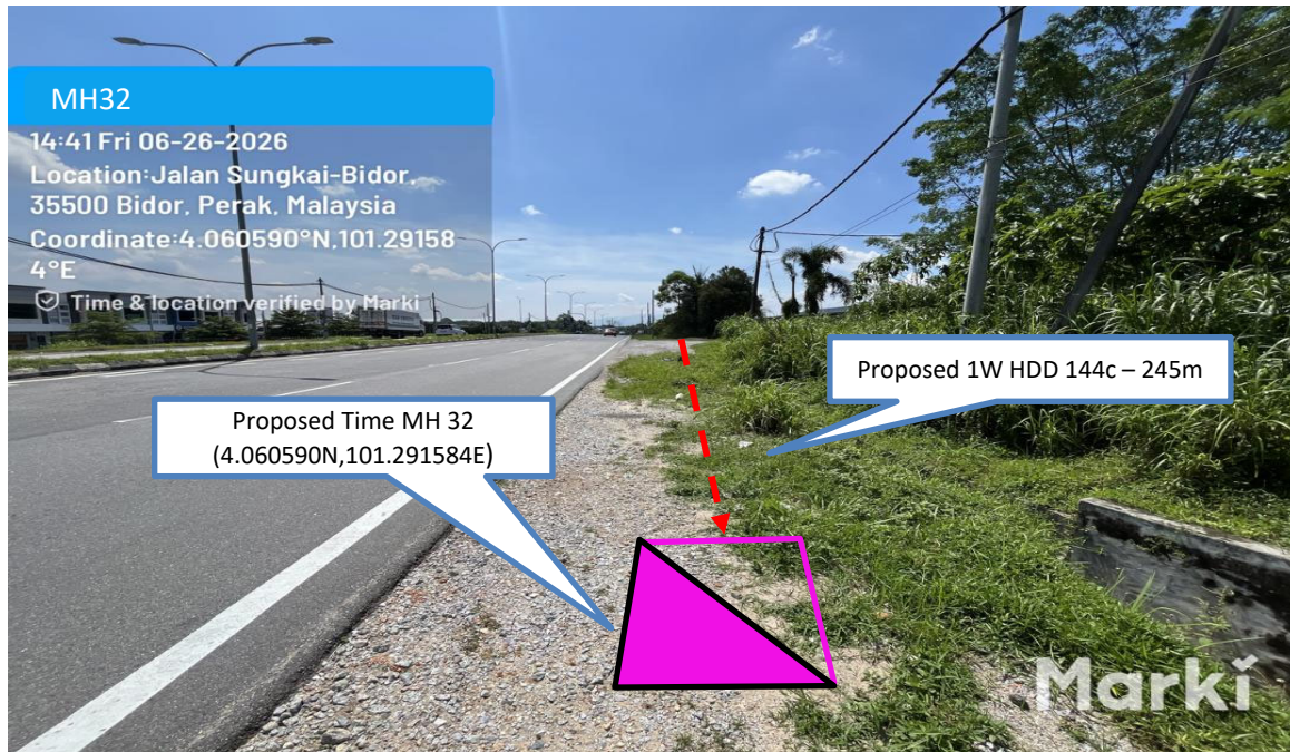
Prop 1W HDD 144C from Proposed Time MH31 to Proposed Time MH32– 245 m
