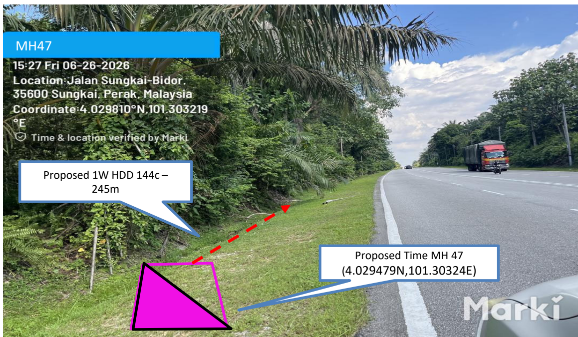
Prop 1W HDD 144C from Proposed Time MH47 to Proposed Time MH48– 245 m
