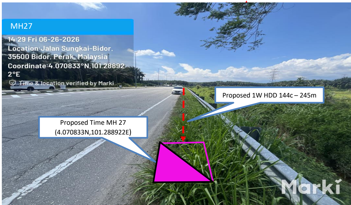
Prop 1W HDD 144C from Proposed Time MH26 to Proposed Time MH27 – 245 m
