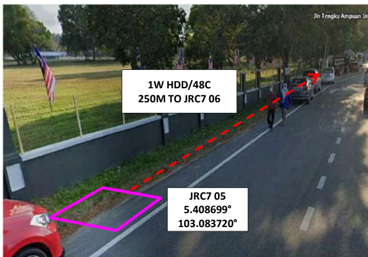
Propose route across Jalan Tengku Ampuan Intan Zaharah - HDD method
