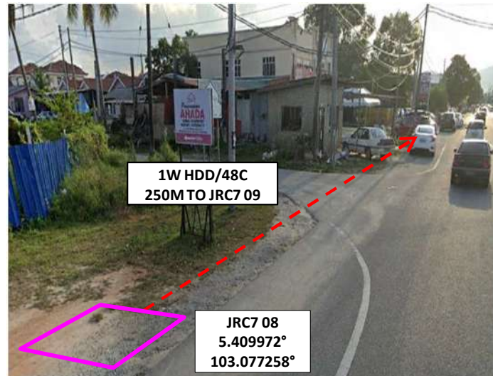
Propose route across Jalan Tengku Ampuan Intan Zaharah - HDD method
