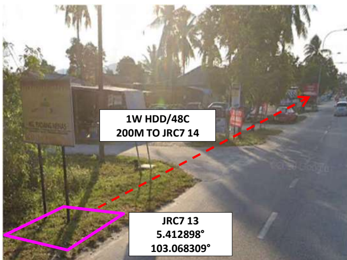
Propose route across Jalan Tengku Ampuan Intan Zaharah - HDD method
