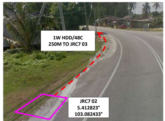
Propose route across Jalan T15 - HDD method
