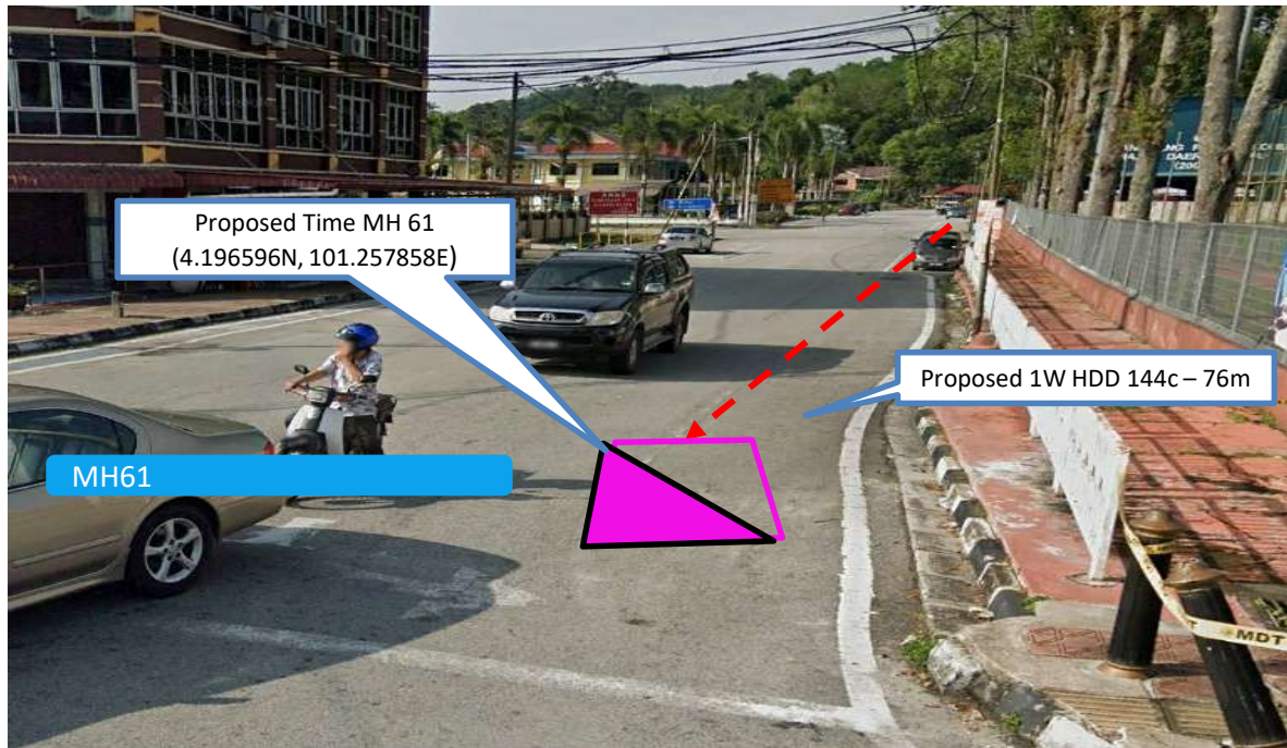
Prop 1W HDD 144C from Proposed Time MH60 n to Proposed Time MH61– 76 m
