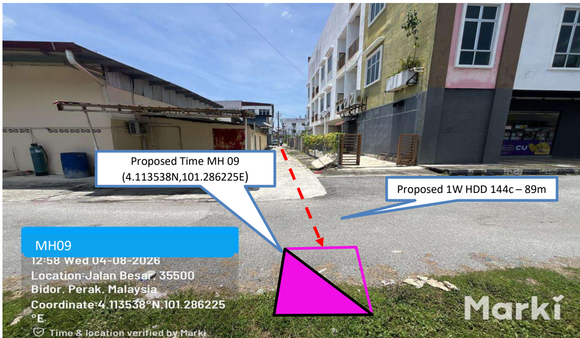
Prop 1W HDD 144C from Proposed Time MH08 n to Proposed Time MH09 – 89 m
