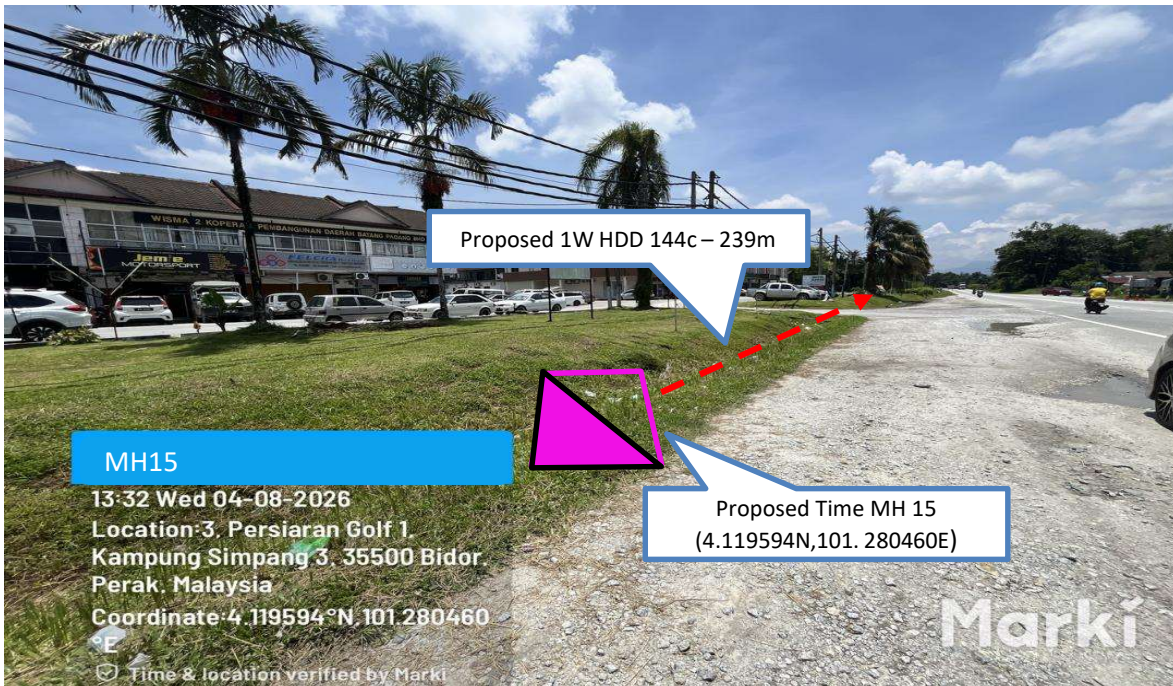
Prop 1W HDD 144C from Proposed Time MH15 n to Proposed Time MH16 – 239 m
