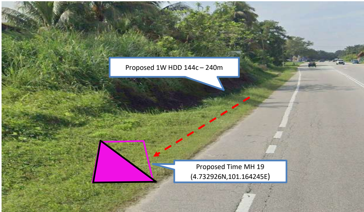
Prop 1W HDD 144C from Proposed Time MH18 n to Proposed Time MH19 – 240 m
