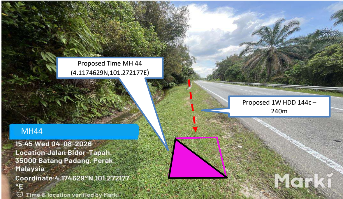
Prop 1W HDD 144C from Proposed Time MH43 n to Proposed Time MH44–240 m
