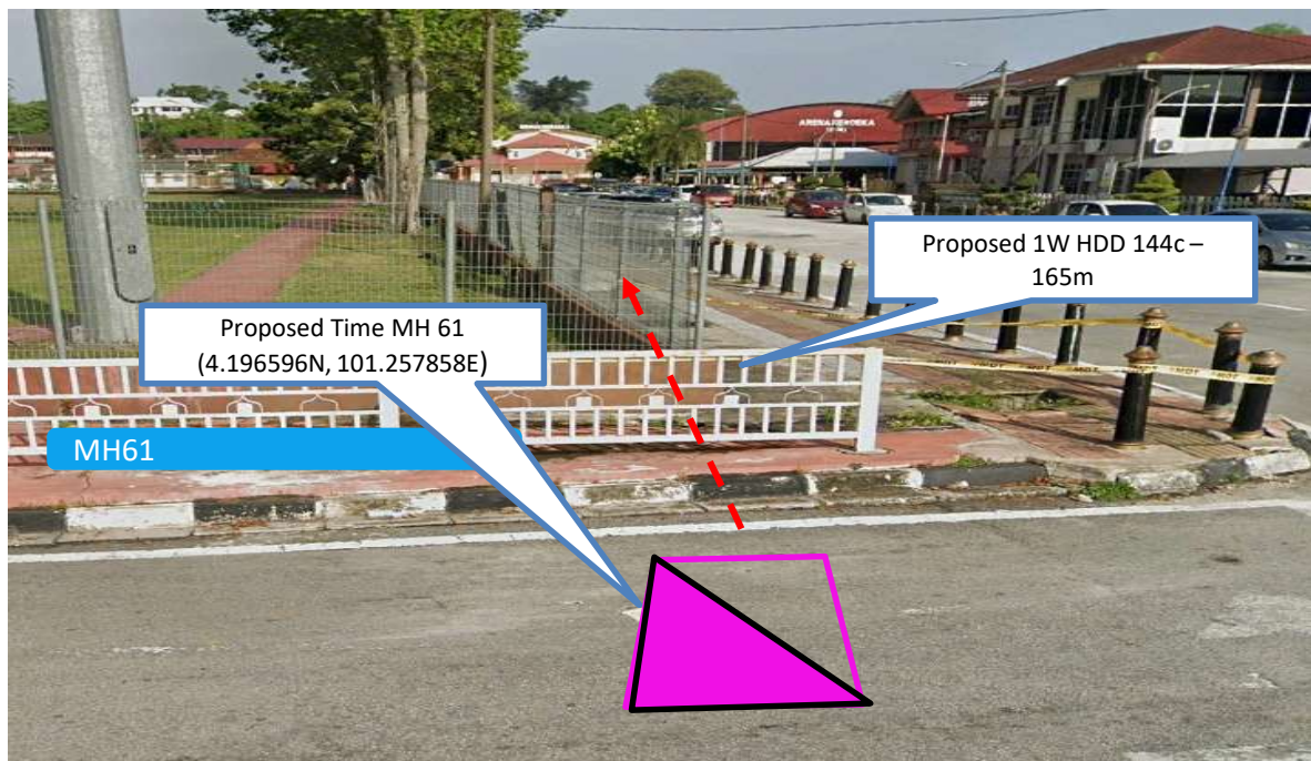
Prop 1W HDD 144C from Proposed Time MH61 n to Proposed Time MH62– 165 m
