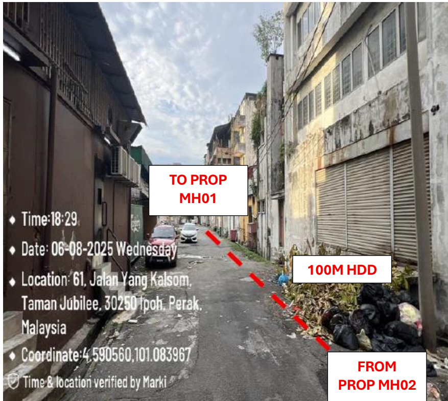
PICTURE 5 : PROPOSE 100M HDD TO PROP MH01
