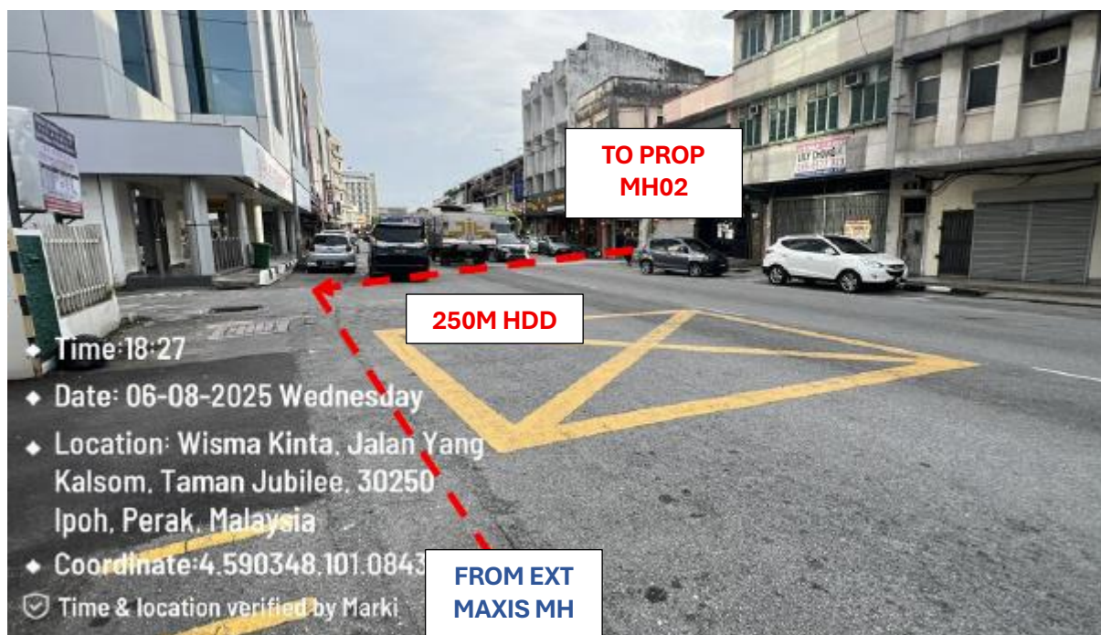
PICTURE 2 : PROPOSE 250M HDD TO PROP MH02
