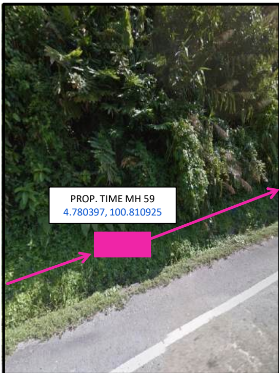
Proposed HDD 1 Way and Pulling Cable 144C from Prop. TIME MH59 to Prop. TIME MH60 at Kampung Pasir Besar
