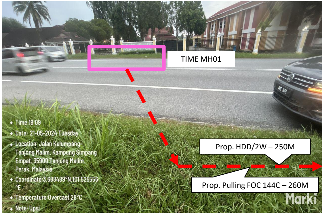
Proposed HDD/2W (30M) and pulling FOC 144C (40M) from TIME MH01 to Prop New TIME MH02
