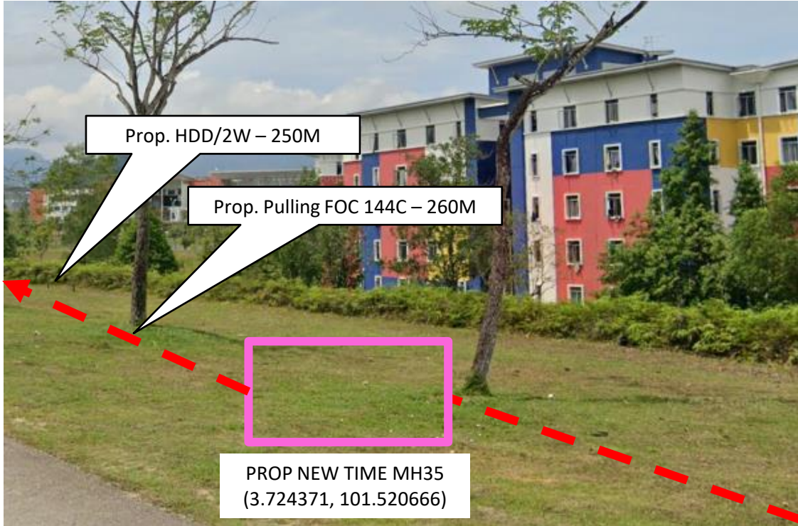
Proposed HDD/2W (250M) and pulling FOC 144C (260M) from Prop New TIME MH35 to Prop New TIME MH36
