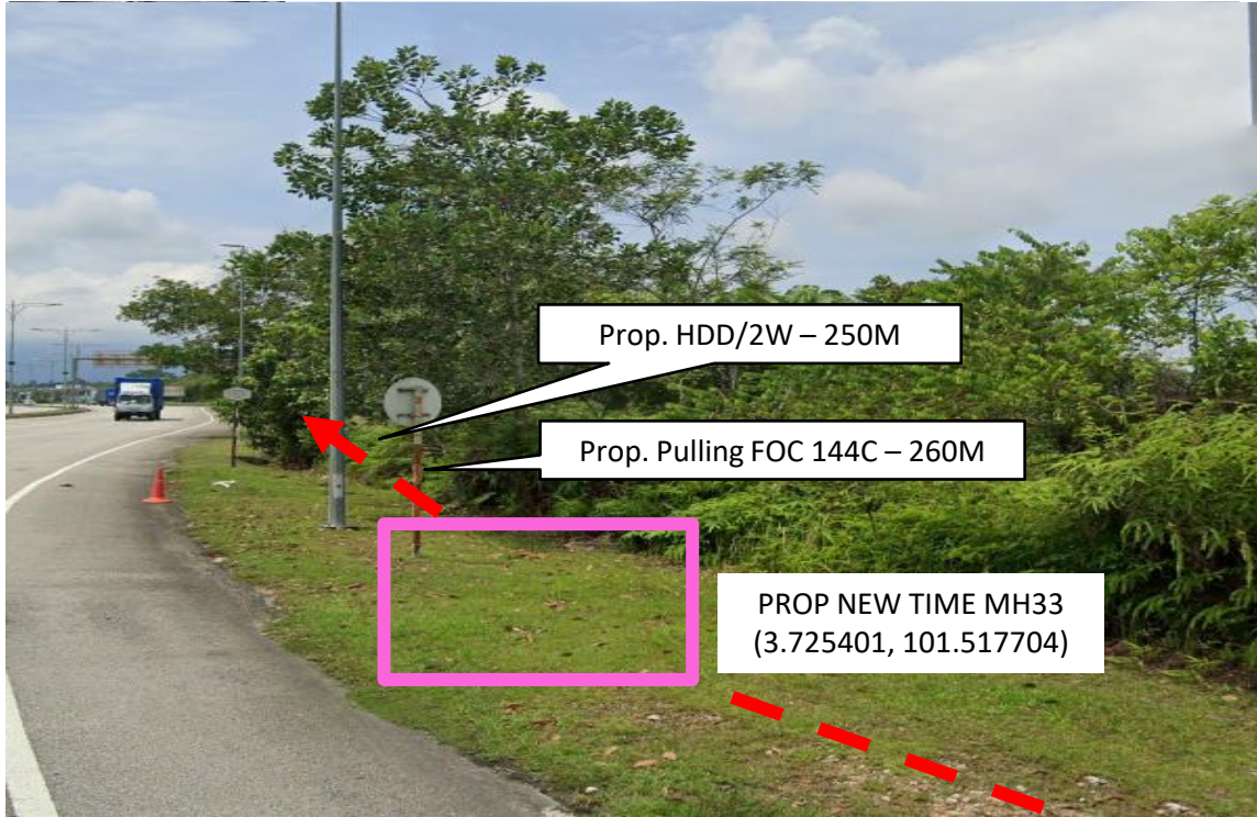
Proposed HDD/2W (250M) and pulling FOC 144C (260M) from Prop New TIME MH33 to Prop New TIME MH34
