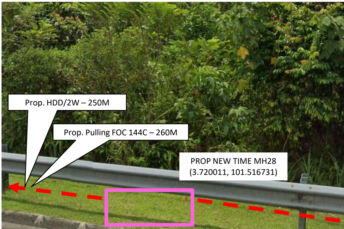
Proposed HDD/2W (250M) and pulling FOC 144C (260M) from Prop New TIME MH28 to Prop New TIME MH29
