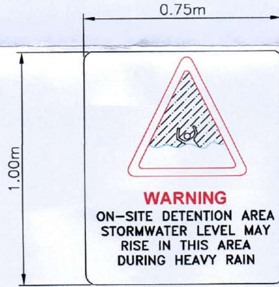
TYPICAL OSD ADVISORY SIGN (UPRCT, 1999) SCALE : NTS Colours: Triangle and "WARNING" - Red Water - Blue Figure and other lettering - Black
