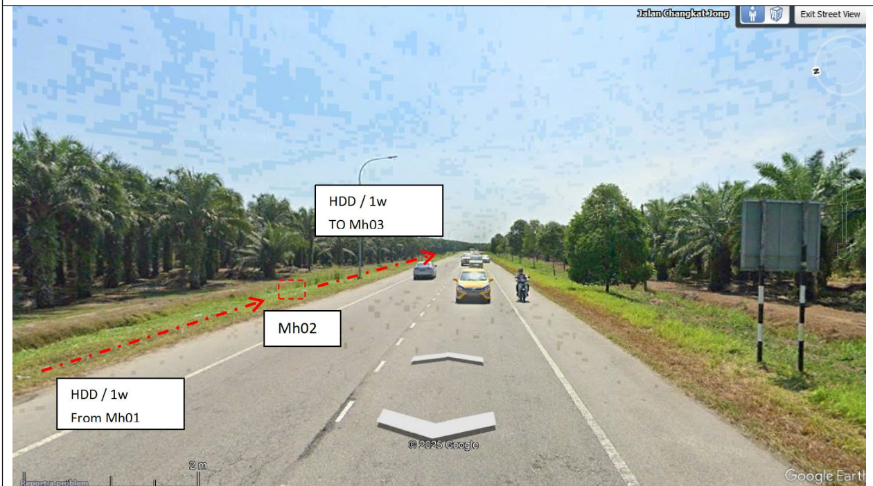
Propose route with 1w HDD GV along Jalan N58 (Jalan Changkat Jong)
