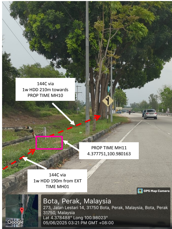
PROP TIME MH11 and prop 1w HDD to PROP TIME MH10 at Ipoh – Lumut Highway (JKR)
