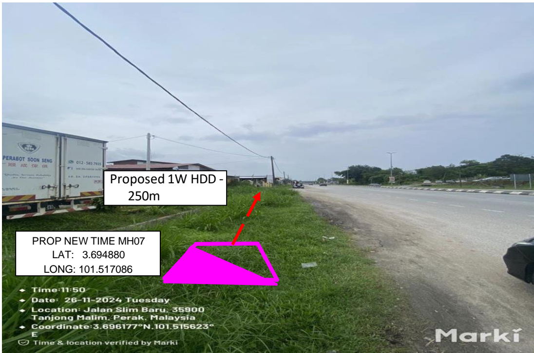
Proposed 1 Way HDD– 250m from Prop New TIME manhole 07 to Prop New TIME manhole 08
