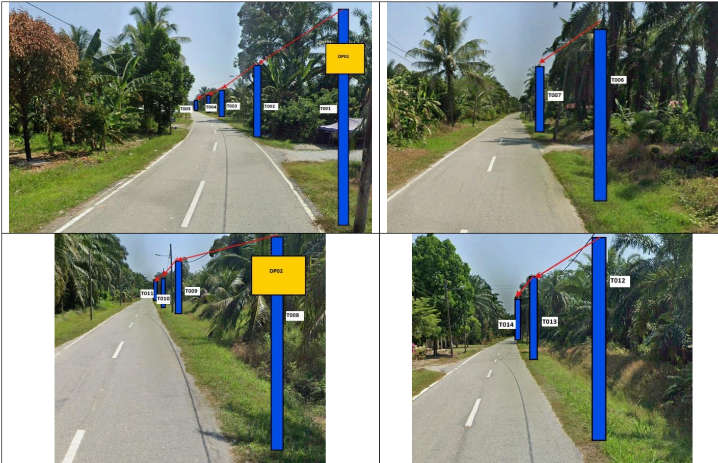
Site Photos – Proposed to install pole 7.5m
