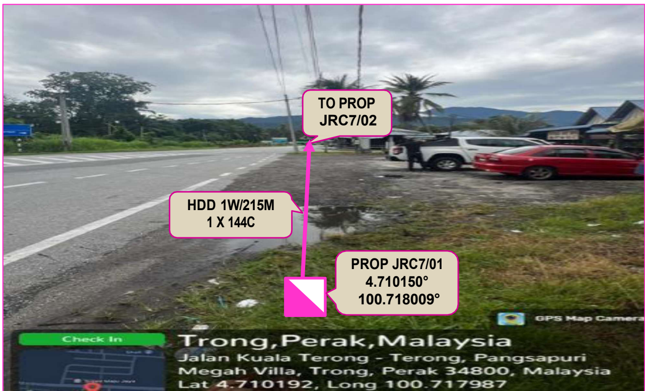
PROP 144C CABLE ROUTING VIA PROP JRC7/01 AT JALAN KUALA TRONG (ROADSIDE)
