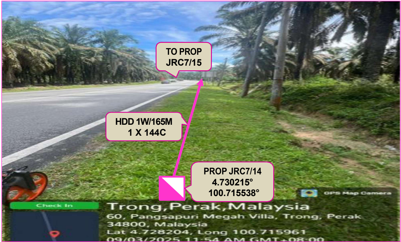
PROP 144C CABLE ROUTING VIA PROP JRC7/14 AT JALAN BESAR (ROADSIDE)
