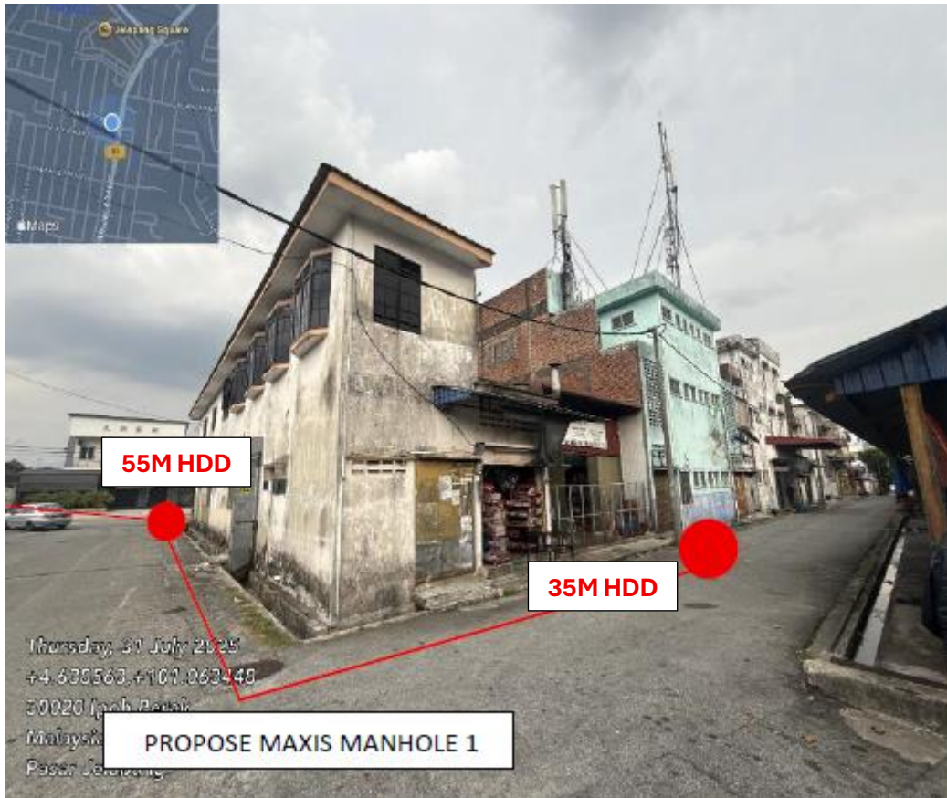
PICTURE 7 : PROPOSE 250M HDD TO PROP MH01
