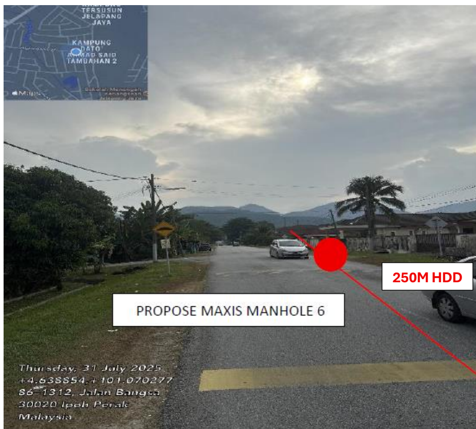
PICTURE 2 : PROPOSE 250M HDD TO PROP MH06
